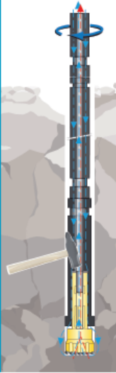
REVERSE CIRCULATION DRILLING
